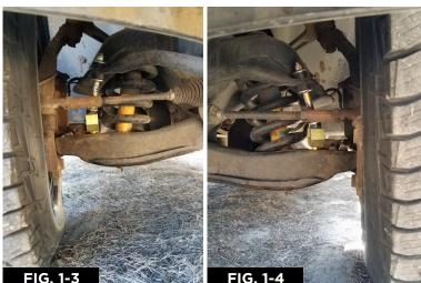
rotate as needed to center lower concave /convex bushings. Hold MAXXLink in place and torque retaining nut to 60 ft/lbs. See FIG 1-2
