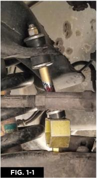
Again, Thank you for your purchase! Enjoy your SuspensionMAXX leveling system! Questions? E-mail us at tech@suspensionmaxx.com or call 1.888.629.9226 4. Install supplied lock washer and start retaining nut Continue on opposing side. Install upper sway bar bushing, washer and nut. Tighten to lightly compress bushings (tighten so approximately 1/4" - 3/8" threads exposed) See Recommended Compression Guide. View MAXXLink and
