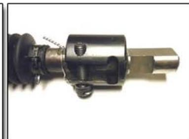
41. Place the upper end of the steering extension into the firewall shaft, install the factory bolt, and tighten to 25 ft lbs. (Fig 4.41)
