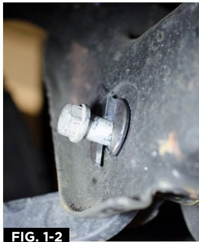
7. Continue holding bracket in place & insert included bolt through both the hole in the bracket as well as the back side of the crossmember.
