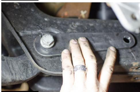
8. From the front side of the crossmember, insert sleeve over the bolt and into the crossmember. See **FIG 1-5 & FIG 1-6**
