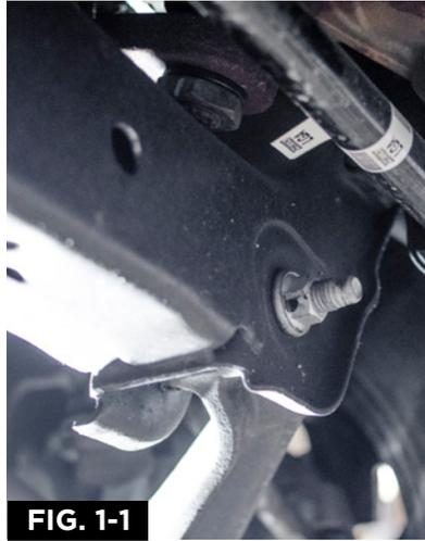
4. Carefully back bolt out a 1/4-1/2 inch using a rubber mallet. **DO NOT FULLY BACK OUT BOLT!**
